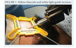
now happens automatically, with the robot recognizing a yellow tensioner from a distance and then homing in on the fiducials as it moves closer to the scalp, eliminating the time needed for the extra step (Figure 1).
